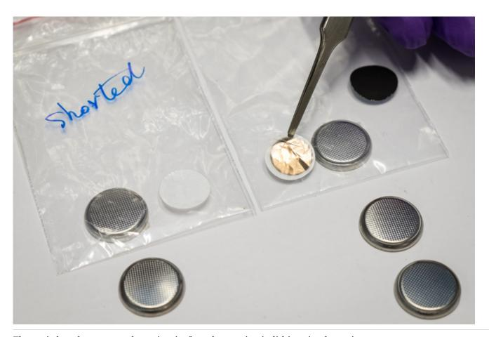
The anti-short layers stop short circuits from happening in lithium-ion batteries.
